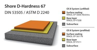
As a rule floor slabs in contact with the ground are not subjected to extreme dynamic stress like intermediate or open-air decks. Besides the resilience, here the requirements are the protection against aggressive substances that damage reinforced concrete, against rising damp, the visually user-friendly colored design and finally the non-slip quality.
